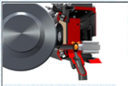
The optional, high-performance valve ensures quick and efficient emptying of ink/coating fluids from the chambers
